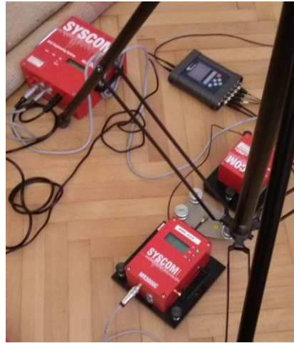
Figure 5 - Vibration measuring system with triaxial acceleration sensor based in the center of the room below dummy head measurement system
